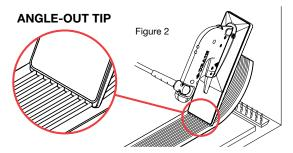
**Angle-Out Tip:** The sole plate has an angle-out tip at the back, this feature will prevent "dragging-off" the hot melt adhesive, especially in doorway situations where the iron is removed by angling it up and out.
